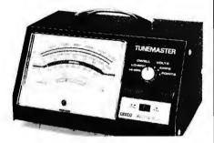
pass); voltage-loss test; ballast resistor test; spark-plug wire test: capacitor test: alternator test; and fuse test. The large 6" (15.2-cm) meter has multi-range, color-coded scales. Controls include a cylinder selector switch and a mode selector. The tester operates on power from the vehicle's battery. The instruction manual provided with the instrument details step-by-step tune-up information for all domestic and foreign cars. \$49.95.
